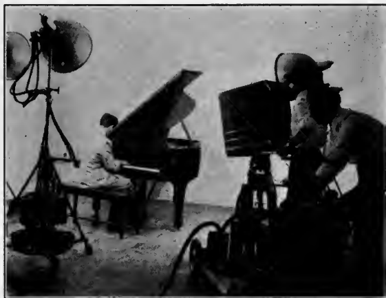
FIG. 18. Scene being televised with cool light from water-cooled quartz mercury arc lamp, in G-E Television Studio, Schenectady, N. Y.
